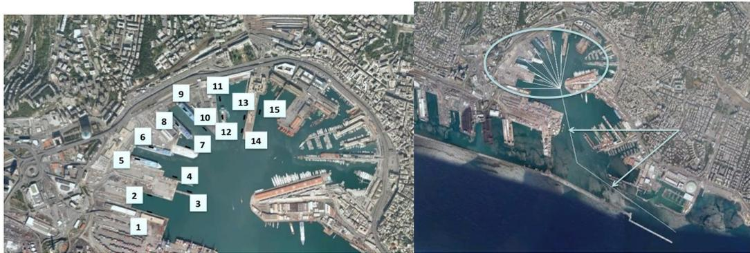
**Fig. 2.2.2.1** – Passenger ships emission sources in Genoa area simulations. On the left ships in hoteling phase, on the right ships in maneuvering phase.
