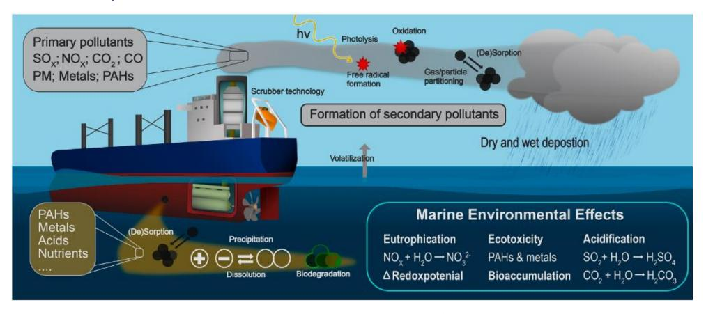
The resulting scrubber discharge water is a chemical cocktail of acidifying, eutrophying and contaminating substances and elements  $\Rightarrow$  toxic cocktail
