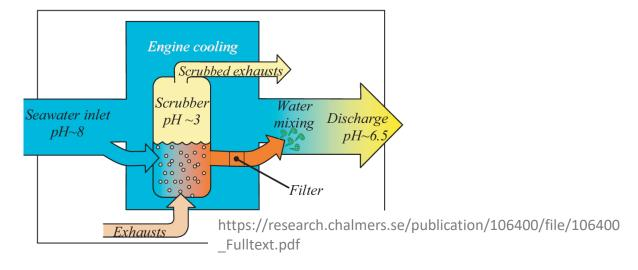
alkalinity measurements showed a significant drop of alkalinity in OL systems (inlet values in the range of 1.6–2.6 mmol  $L^{-1}$  and outlet values between 0.0 and 1.4 mmol  $L^{-1}$ ). in CL systems, alkaline substances are added to the fresh water to adjust the pH level. It has been reported zero (0 mmol  $L^{-1}$ ) alkalinity in all discharge water samples from CL systems.
